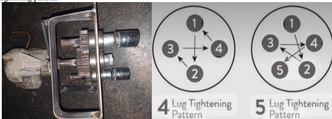
FIGURE 1: Multi-nut lightener and lug tightening pattern
