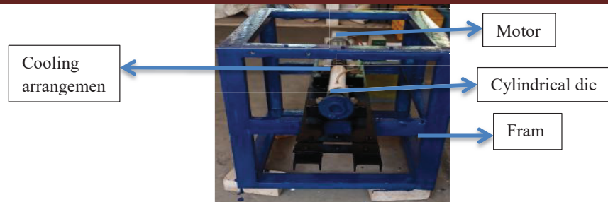
FIGURE 4. a)Horizontal centrifugal casting machine
