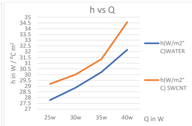
FIGURE 8. Heat transfer coefficient vs heat input
