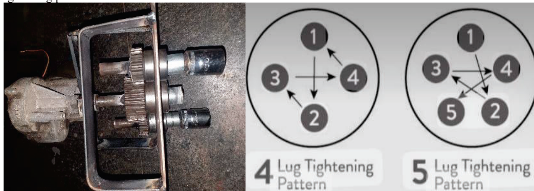
FIGURE 1: Multi-nut lightener and lug tightening pattern
