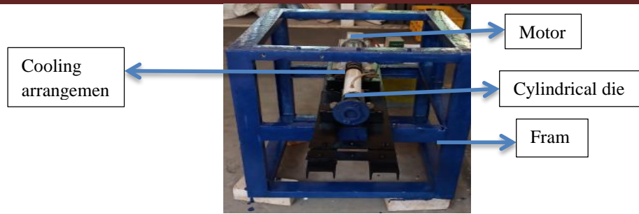
FIGURE 4. a)Horizontal centrifugal casting machine
