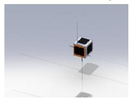
will link to a number of LEO satellites and ground stations using the Automatic Position Reporting System (APRS) protocol. This will allow remote access for worldwide position/status reporting using simple mobile radios with omni-directional antennas. Real time position reporting is accomplished using GPS data. Duchifat-1 will be capable of transmitting a variety of data including short text messages and telemetry data acting as a digipeater. The APRS protocol is useful for SAR (Search and
