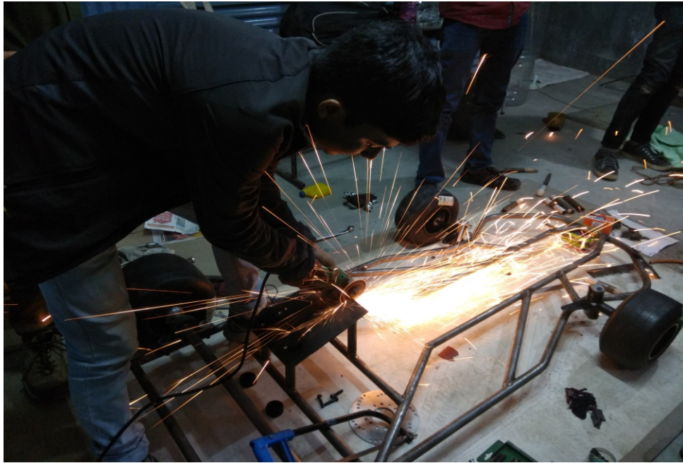
Photograph 1 : Adding support to Engine Mount
